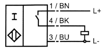
Fig. 5.1: Proximity switch wiring scheme
